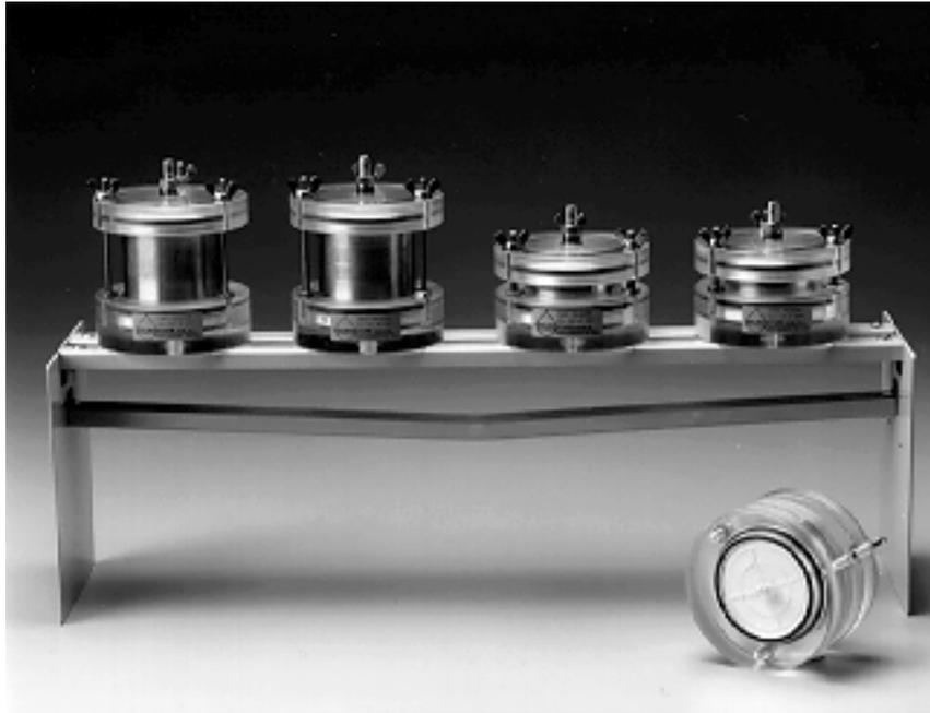
*Fig. 1a 1400 Tempe Pressure Cells with 3cm cylinders and 6cm cylinders) mounted on the Tempe Cell Stand*
