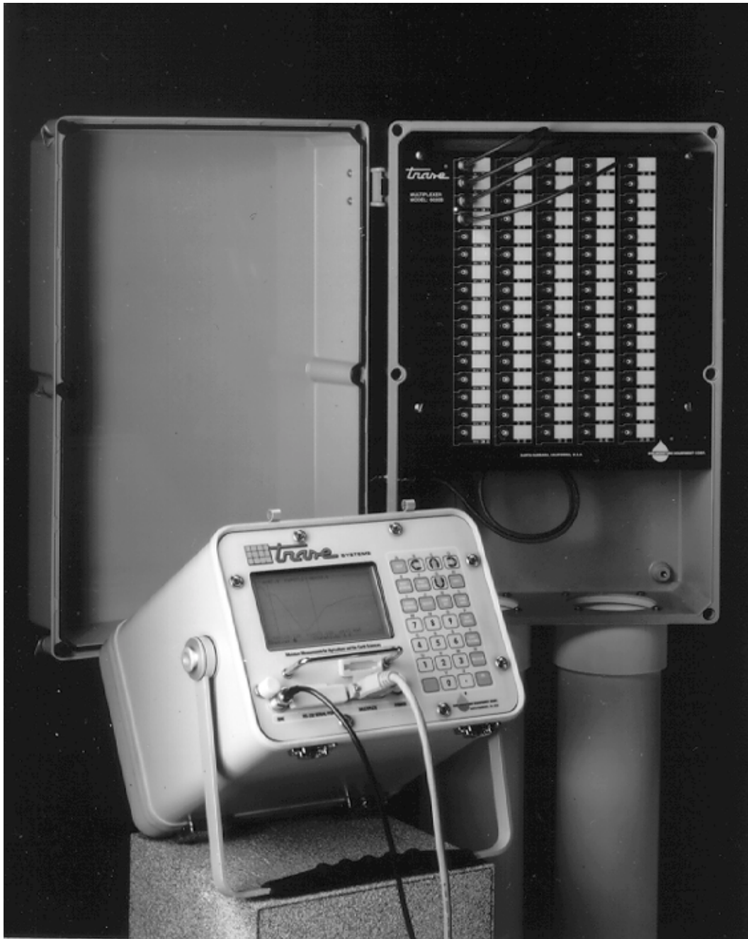
Figure 1 - Trase Unit and Multiplexer Enclosure
