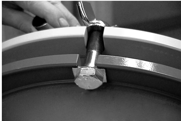
Fig. 7 - Clamping Bolt Heads properly placed into constraining groove. Note the square head fitting into the clamping ring
